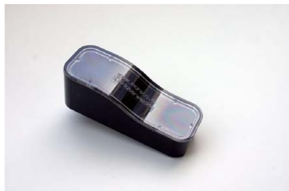
Fig. 5: 3D welded sample, highly pressure-tight up to 5.5 bar
