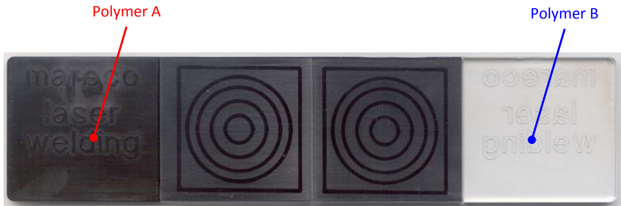
Figure 4: laserwelding test-strip Polycarbonate/Polycarbonate (source: Mareco Kunststoffen 2006)
